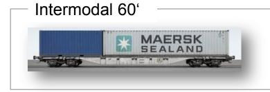
The most flexible "allround" railcar for combined transportation with an ideal loading weight of 70 t. Excellent for maritime containers, tank containers and swap-bodies.
