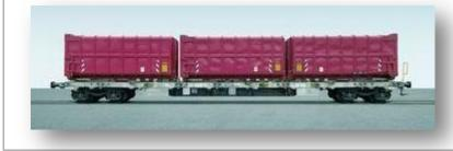
The ACTS System (Roll-off Container Transport System) can be used on almost all loading tracks with hard surface road access. The standard rolloff containers can be pushed/pulled between wagon and truck in a singleman operation by means of a chain or hook system.
