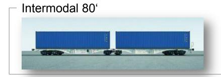
With a loading length of 80 feet this container car is ideally suited for the transport of 20' and 40' containers. With its high cargo weight of 107 t and its loading length, the Sggrss 80' provides the ideal weight/ loading length ratio.
