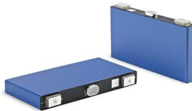
A prismatic design indicate a flat battery design. The stacks can be wound (as shown in the photo) or stacked (with alternating cathode/separator/anode structure). The stacks are usually inserted into rigid casing to form prismatic.
