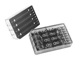
State-of-the-art array containing over 200,000 femtoliter-sized wells and integrated microfluidics.
