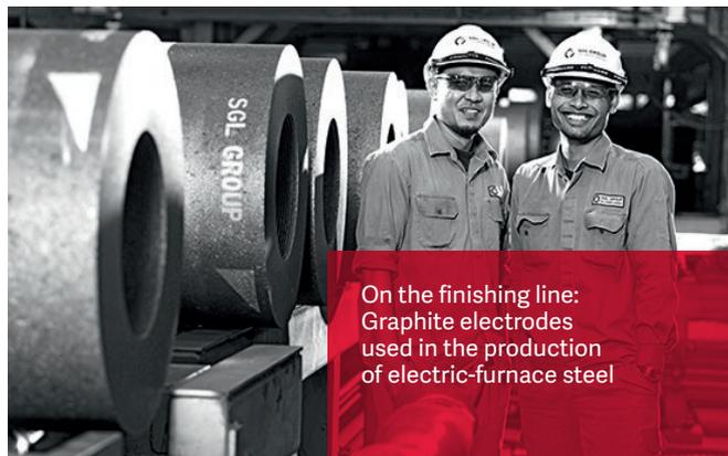
On the finishing line: Graphite electrodes used in the production of electric-furnace steel
