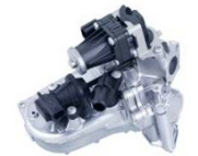
Valve, cooler, bypass and bypass actuator
