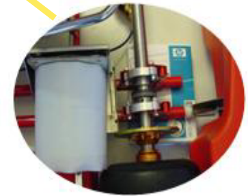
Motor control Inverter stage with HybridPack1 TC1796 starter kit
