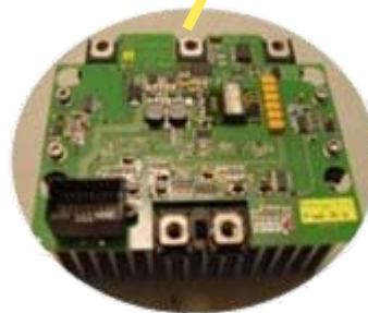
Motor control Inverter stage with HybridPack1 TC1796 starter kit
