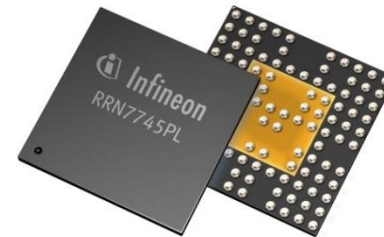
77 GHz radar IC in eWLB package
