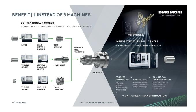
These benefits can be increased, in particular, by combining the machine tool with automation and digital tools. We offer a standard or customized automation solution for almost every DMG MORI machine or application. This allows existing resources to be used in an effective and sustainable way.
