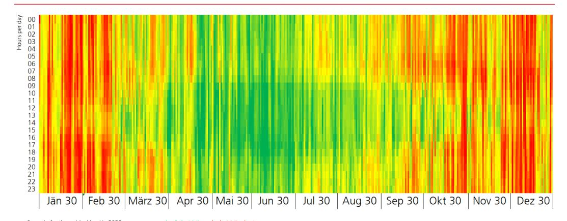
Scenario for the residual load in 2030; green: oversupply of electricity; red: electricity shortage
