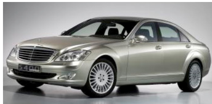
• S 400 BlueHYBRID (first PC with lithium-ion battery)
