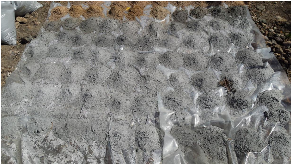
Figure 1 – RC samples from recent drilling at Epanko
