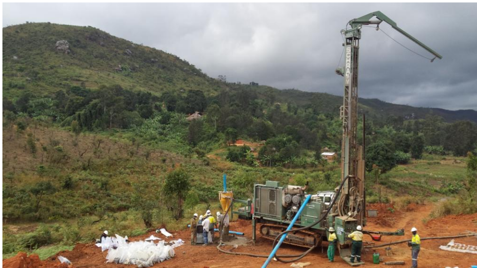
Figure 2 – RC drilling at Epanko Deposit
