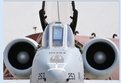
Cobalt-based superalloys are used in jet engines—including military fighter jet aircraft—because of their stability at high temperatures. Photograph courtesy of the U.S. Air Force.
