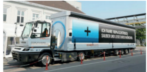
BMW's 40-ton electric semi-truck, with 100 km rang, currently in service (Germany)
