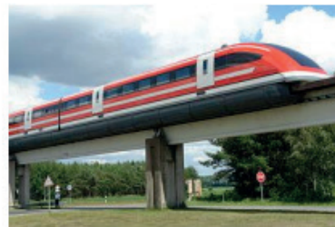
Transrapid 09 Maglev train, designed for speeds up to 500 km/hr (Nd, Pr, Tb, Dy)
