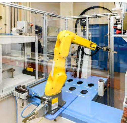
**This robot analyzes stamping samples fully automatically.**
