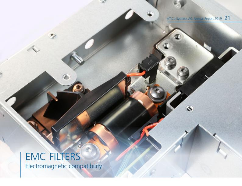
The rising number of appliances that produce and use energy is increasing demand for EMC filters for electromagnetic suppression. Unwanted interference between appliances can degrade performance of the power supply and onboard systems. Therefore, it has to be suppressed to prevent unwanted disruption.
