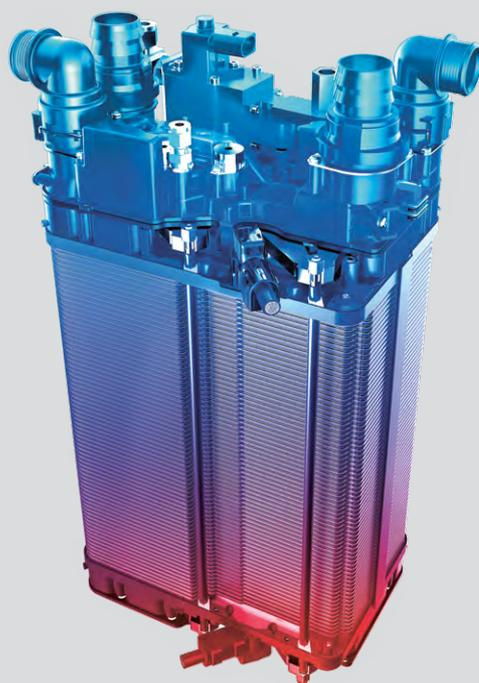
The image on the cover depicts an ElringKlinger fuel cell stack consisting of metallic bipolar plates, membrane electrode assemblies, seals, and end plates as well as a tensioning system. The plastic media module performs important system functions by integrating sensors, valves, and water management, for example.
